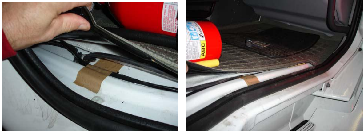
Figure 27 Sample Cable Placement in a Vehicle Cab
